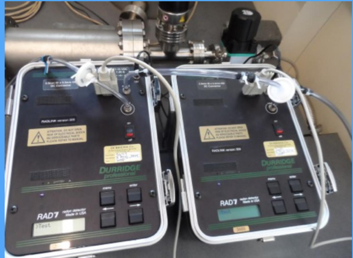
Fig. 3 - Two DurrIDGE RAD7s set up in series with the 2.7 l vessel
